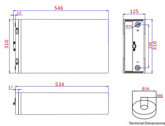
48V system: Total installation depth 546mm, including connector, bolt, insulation protective cover.
